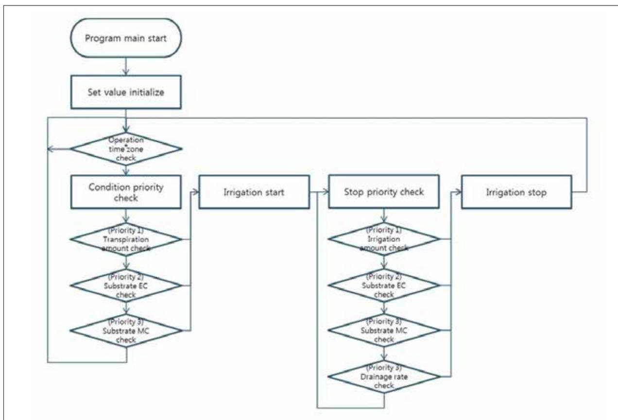
Figure 6. Flowchart of an irrigation control.
