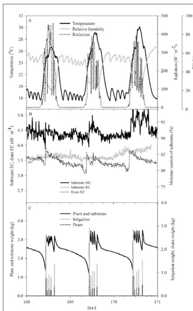
Figure 2. Aerial environmental parameters [temperature, relative humidity, and radiation, (A)], root-zone environmental parameters [substrate moisture content and electrical conductivity (EC), and drainage EC, (B)], and weights [irrigation amount, drainage amount, and weight changes of plant and substrate, (C)] measured in Treatment 2 (168–170 DAT, days after transplanting).
