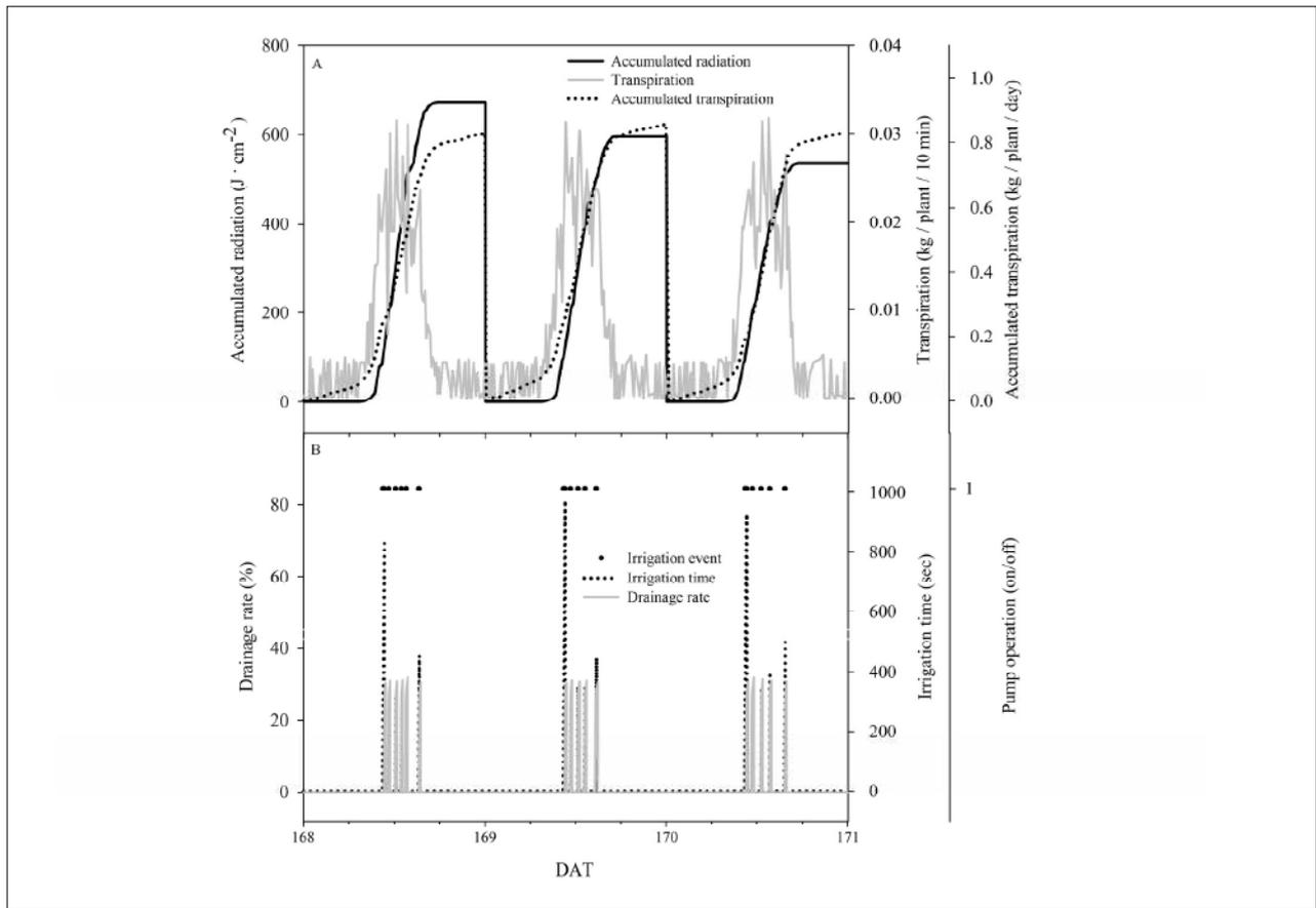
Figure 3. Accumulated radiation, calculated transpiration, and accumulated transpiration (A), and pump operation, irrigation time, and drainage rate (B) in Treatment 2 (168-170 DAT, days after transplanting).
