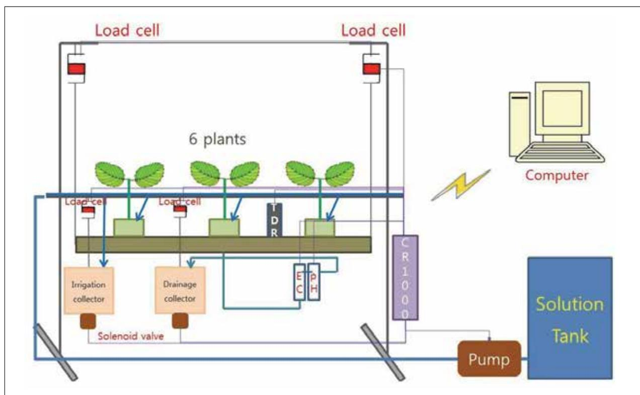
Figure 1. A schematic diagram of the irrigation control system used in this study.
