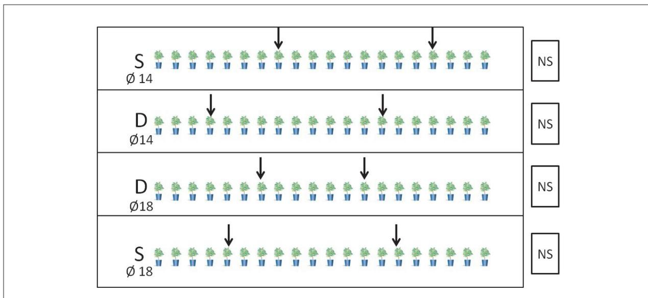
Figure 1. Experimental layout (one replication) was defined by a factorial combination of two irrigation systems: drip-irrigation (D) or subirrigation (S) and two pot dimensions (14 or 18 cm in diameter). Each replication consisted of one bench containing 20 plants. The nutrient solution (NS) was pumped from independent tanks having a volume capacity of 60 L. In each replication, two tensiometers (arrows) were installed to provide a representative reading of the substrate moisture tension.
