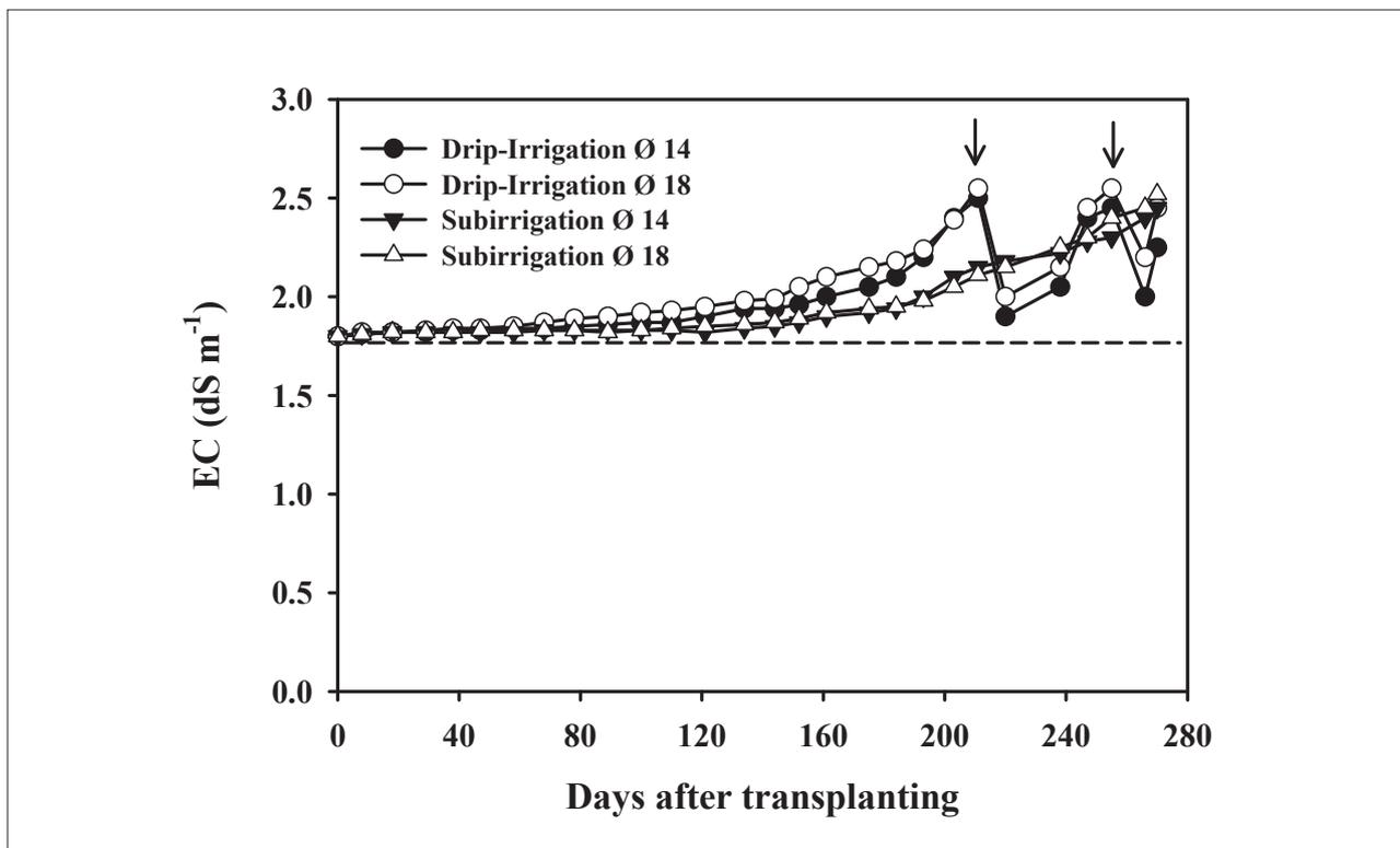
Figure 3. Changes in the electrical conductivity (EC) of the recirculating nutrient solution as affected by pot size and irrigation system of *Murraya paniculata* grown during the 2011–2012 season. The arrows indicate when the EC exceeded the threshold values of 2.5. The EC of the solutions was restored to the target value by adding water.
